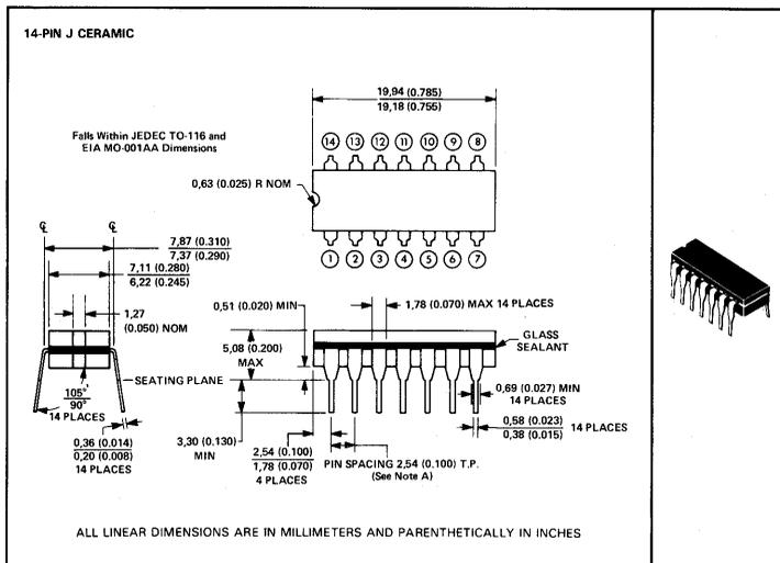
NOTE A: Each pin centerline is located within 0,25 (0.010) of its true longitudinal position.
